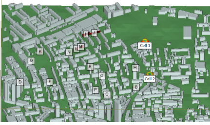
Fig. 8. 3D model of a London area, location of cell sites, and potential RIS sites.
